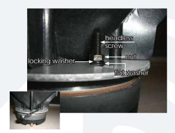
Four nuts and eight washers may be removed from the driver. removed from the driver using the 8mm open end wrench. Turn counterclockwise to loosen and remove, clockwise to tighten. The other three are located around the horn assembly. Lift the horn up as the nuts are loosened. It cannot be removed otherwise. Notice that the flat washer is on the bottom, followed by the locking washer, and finally the nut.
